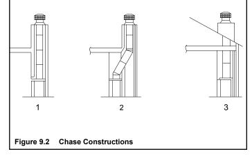
**WARNING!** You must install false ceilings and ceiling firestops at each floor of the chase or every 10 ft (3.05 m) to control spread of fire.
